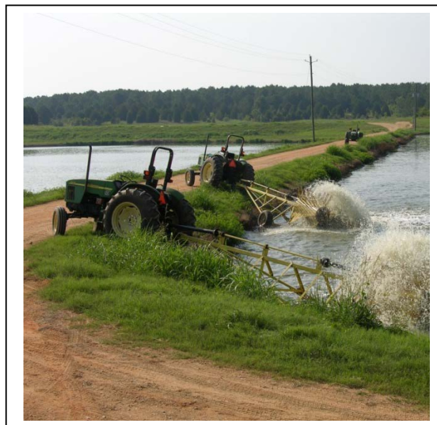
Figure 10 Tractor-driven emergency paddle wheel aerators.
