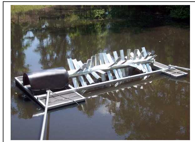
Figure 7 Electric paddle wheel aerator. 1
