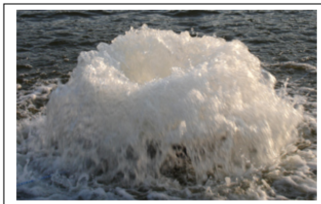
Figure 4 Float-mounted vertical pump aerator in operation.
